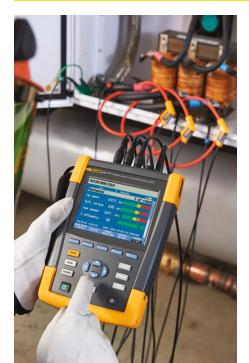
Power Quality monitoring in compliance with EN 50160 at Main Incomer. Power Quality monitoring at UPS input / output The above includes logging of power and P.Q. parameters such as:
